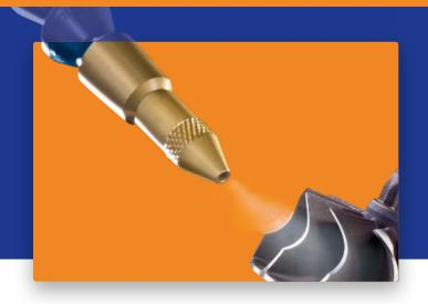
Minimum quantity lubricants, shortened MQL, are applied to the operating range between tool and workpiece by means of special spraying systems. Thus, optimum lubrication and cooling is ensured by minimum consumption of lubricant.
